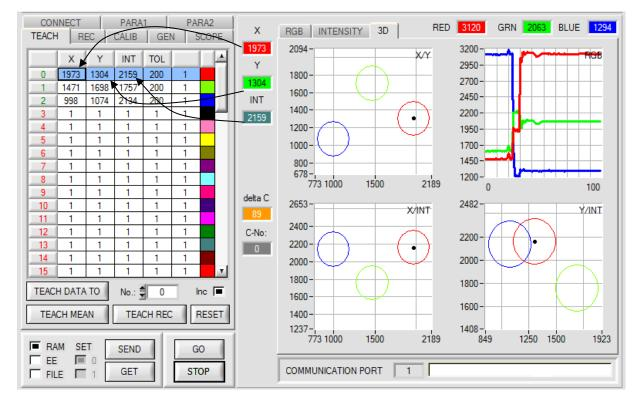
Now press the **SEND** button again to inform the sensor about the taught color. Then activate the **GO** mode again. When the sensor recognises a row vector (color), the corresponding row number is visualised on the software interface under **C-No:** A value of 255 means that none of the taught colors were recognised.
