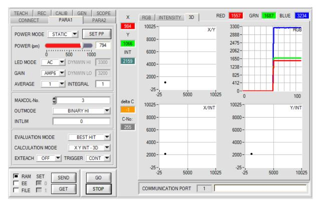
Step 4: An X and a Y coordinate as well as an intensity INT are calculated from the red, green, and blue data. X = (R\*4095) / (R+G+B)Y = (G\*4095) / (R+G+B)INT = (R+G+B) / 3
